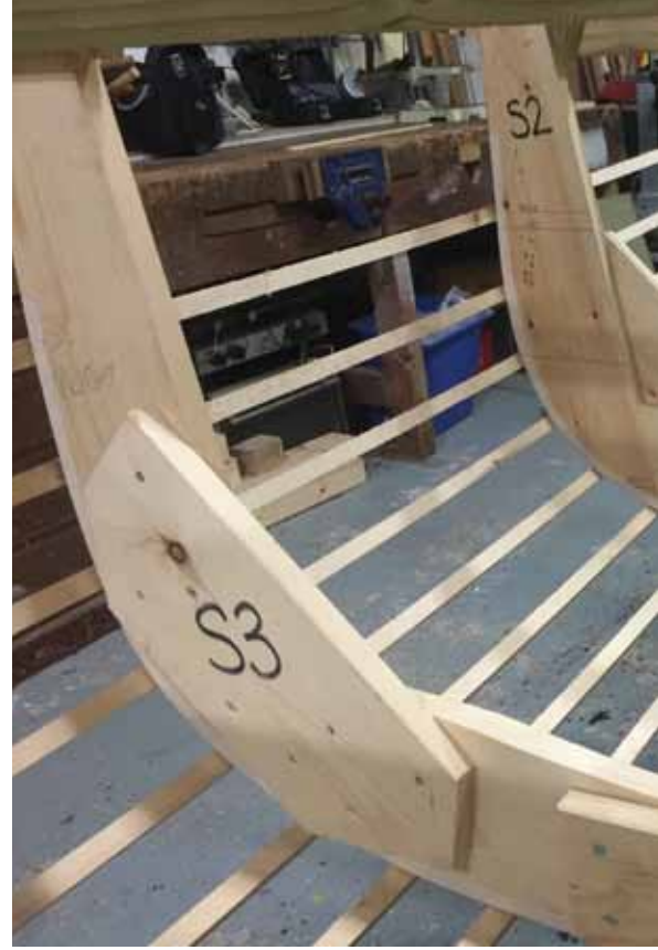
Above left: The little pram required just three building moulds, set up on the hog and braced from a beam above.
