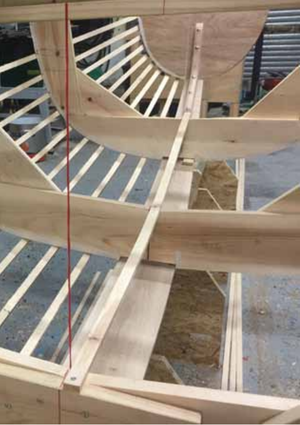
Above left: Finding grown crooks takes forever; jointed knees are also stronger. Below: Fully framed with closely-spaced steamed green oak 'timbers'.
