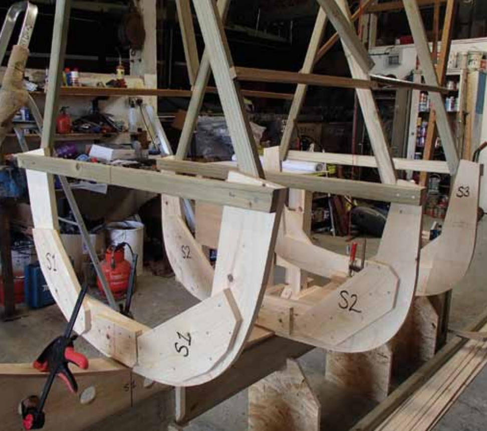
Above left: The little pram required just three building moulds, set up on the hog and braced from a beam above.
