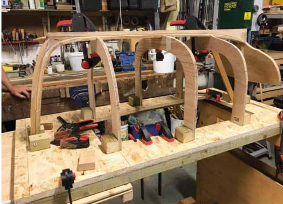
**Above:** *Clinker boats are traditionally built right way up to make riveting the planks and frames easier. Building upside down necessitated a boat-shaped cutout for access..*
