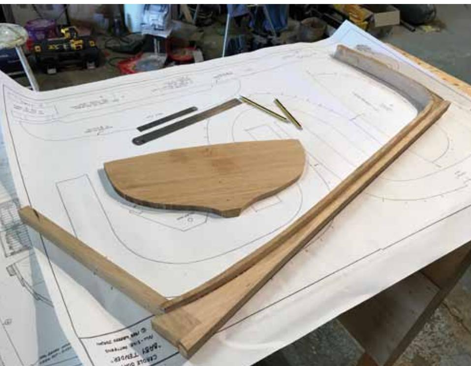
It's always easier to rivet planks single-handed if the boat is built right way up, so to allow working from below, the centre of the building board was removed in a boat shape. The whole baseboard structure was clamped to trestles so the boat could be built comfortably at waist-chest height to save sore knees.
