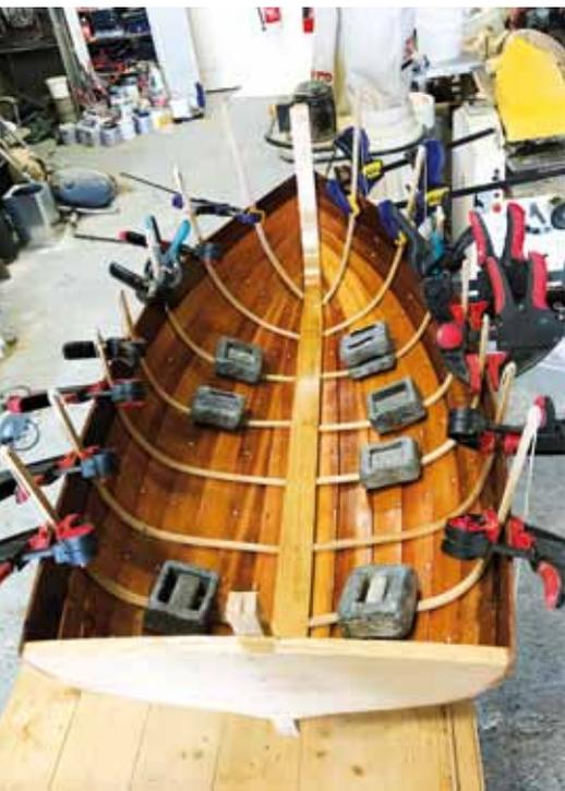
**Above:** *The fully planked hull is lifted off the moulds and turned right way up for...*
